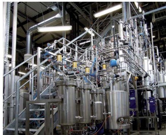
Multifunctional fermentationscascade from 10 l to 10,000 l Bioreactorvolume
